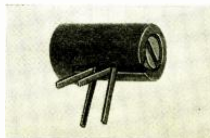
A metal-oxide rectifier. A metallic film provides contact to the oxide. (No. 409)
