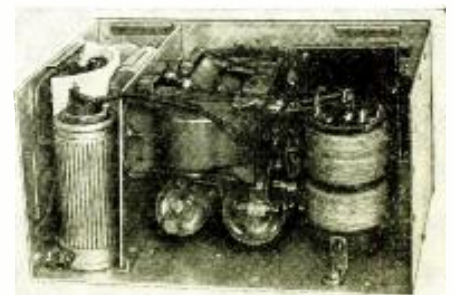
Fig. C The appearance of the oscillator from the back. Note that two tubes are horizontal.
